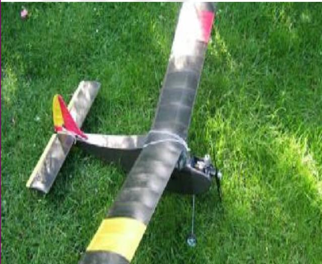
The original plan included two wingspans, 36 and 44 inches by adding wing bays. Many Free Flight modellers chose the 36-inch wing while early R/C'ers (adding rudder and elevator control) chose the 44 inch wing for its greater wing area. The larger model has since grown to 48 inches but with today's super-lightweight servos and receivers, either wing is a viable option.
