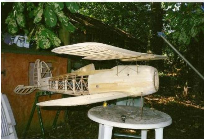
The model is scratch built from plans that John drew up, and is largely finished except for the cowl, canopy, undercarriage, wing spars and covering. It has a wingspan in the region of 8 ft. and will weigh in at about 25lb when complete. Included with the
