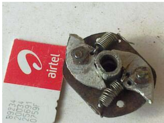
Home Built One Way Bearing
